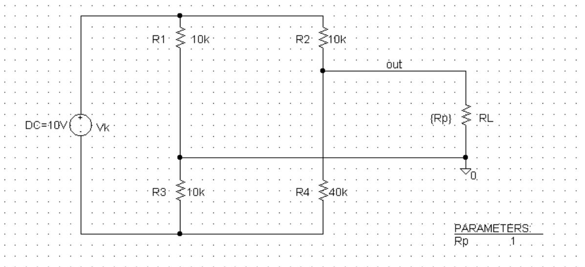
Fig. 1: Bridge circuit with independent voltage source
