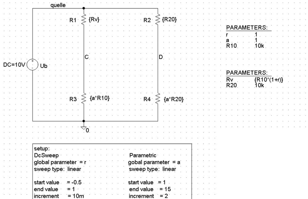
Fig. 3: Bridge circuit for sensitivity analysis
