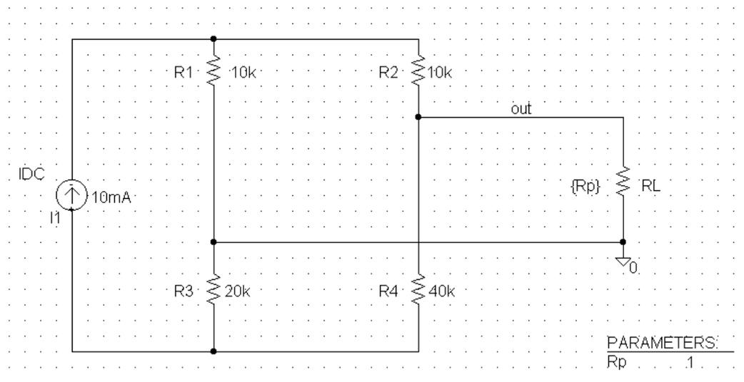
Fig. 2: Bridge circuit with independent current source
